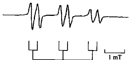
Fig. 4 EPR spectrum of PS-DC, room temperature, [PS-DC] = 0.1 \text{ mol/L} , [MNP] = 0.04 \text{ mol/L}
